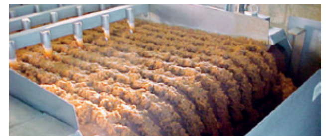
Rows of baffles for sludge draining and distribution.
