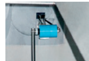
Position sensor for belt tracking
